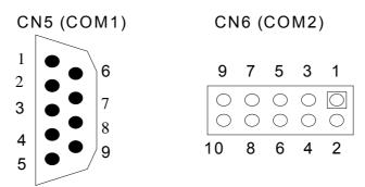
Figure 0-5 CN5 & CN6: RS-232 Connector
